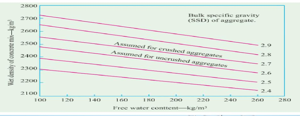
Fig. 3: Relationship between free-water cement ratio and wet density of fresh concrete
